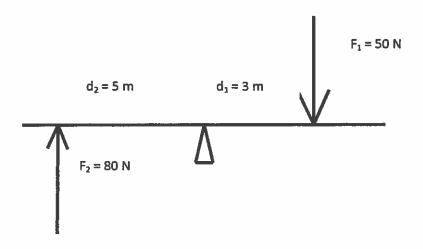
2. Find the net torque on the 15.0-m long lever.
