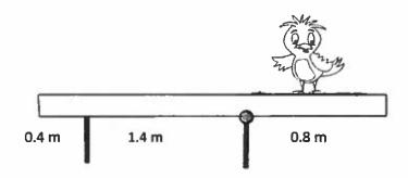
Example: Two people support a plank of length 3.0m and weight 200N as shown below. Their 500N friend is sitting on the plank 1.0 m from the end. Determine the force exerted by each person.
