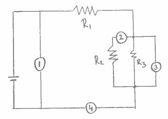
2. What are the potential differences, V<sub>1</sub> and V<sub>2</sub>, in the circuit shown below?
