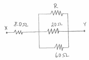
7. The current in the 8.00  $\Omega$  resistor in the circuit below is 0.500 A. Find the current in the 20.00 $\Omega$  resistor. Justify each value by a calculation or Kirchhoff's Rule.
