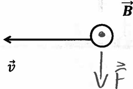
6. Determine the direction of the magnetic field for diagram below, where the force vector represents the maximum magnetic force on a positively charged particle moving with the velocity vector.
