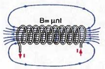
The magnetic field is concentrated into a nearly uniform field in the center of a long solenoid. The field outside is weak and divergent.
