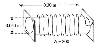
What is the current in the windings that would produce a magnetic field of 0.060 T at the centre of this solenoid?
