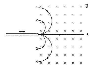
One type of ion is observed to follow path 2. Which path describes the one taken by an oppositely charged ion with twice the mass and twice the charge? (Assume all ions have the same speed.)
