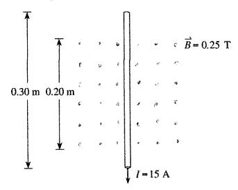
What are the magnitude and direction of the magnetic force acting on this conductor when it carries a 15 A current?
