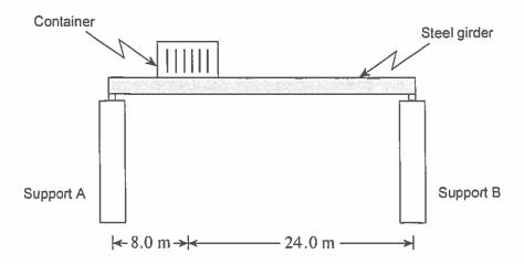
What are the upward forces at the girder end points when it is bearing a 3 700 kg shipping container 8.0 m from support A? (7 marks)
