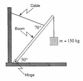
What is the tension in this cable when the boom supports a 150 kg mass as shown? (7 marks)
