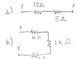
3. Find the a)net resistance, b)electric current, c)voltage drop across resistor 1 and d)voltage drop across resistor 2.
