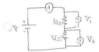
4. Find the electric current and voltage drop across resistor 2. Show proper connection of a voltmeter to measure the voltage drop across resistor 2.
