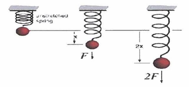
Example 1: Find the force exerted by a spring that was stretched by 50cm and its spring constant is 75N/m.
