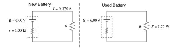
If resistor R now dissipates 1.75 W, what is the internal resistance of the used battery?
