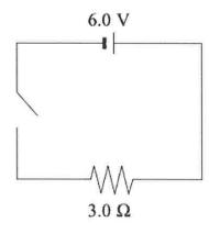
What total charge flows through the resistor if the switch is closed for 40 s?
