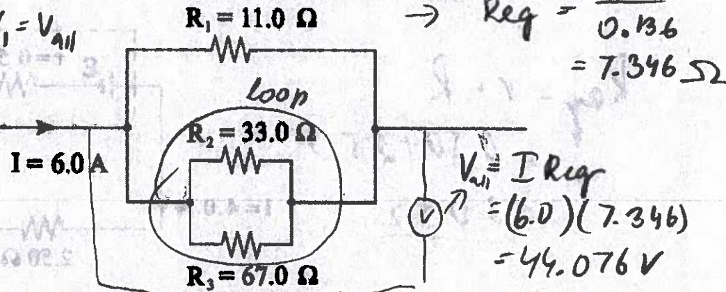
What is the current through resistor  $R_1$ ?
