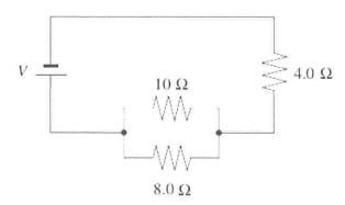
What happens to the power dissipated by the 8.0  $\Omega$  resistor and by the 4.0  $\Omega$  resistor?
