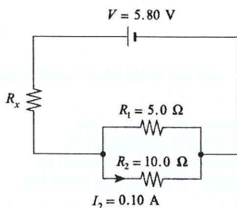
$$V_2 = R_2 I_2 \\ = (10.0)(0.10) \\ = 1.0 \text{ V}$$
