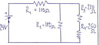
Step 1: locate all resistors in parallel \_\_\_\_\_, and \_\_\_\_\_
