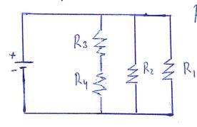
$R_1 = 10\Omega$ ,  $R_2 = 5\Omega$ ,  $R_3 = 8\Omega$ ,  $R_4 = 4\Omega$
