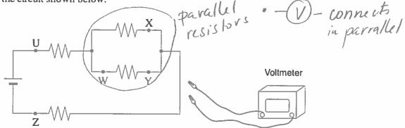
Across which two connection points should the student connect the voltmeter?
