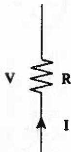
The voltage across the resistor increases from  $V$  to  $2V$ . The resistance remains the same. By what factor has the current changed?
