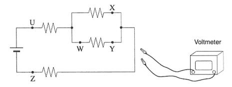
Across which two connection points should the student connect the voltmeter?
