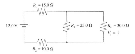
What is the potential difference,  $V_4$ , across the 30.0  $\Omega$  resistor?
